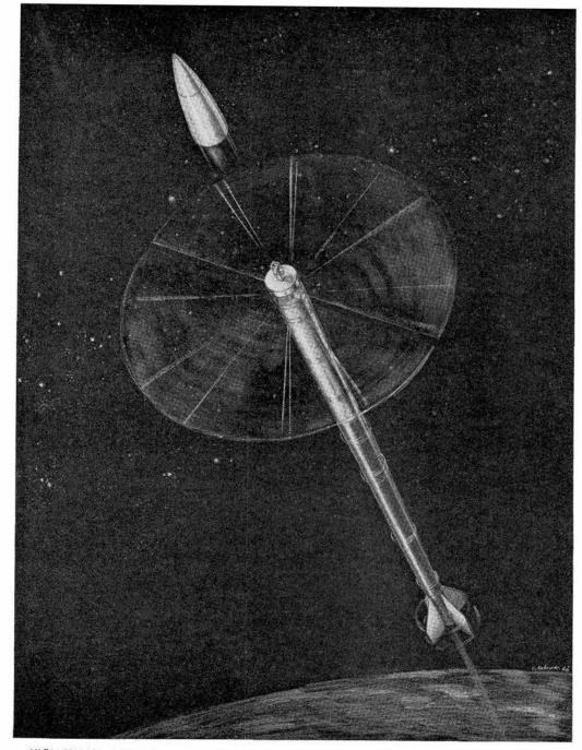
HIGH-FLYING SAMPLER—artist's conception of the Sandia-developed device for sampling the atmosphere above 300,000 feet. The eight-foot diameter mylar disk is shown in its deployed state.
